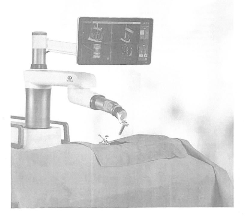
Setup for ExcelsiusGPS<sup>™</sup> involves system draping and simple positioning of the frameless robotic arm. When the procedure is complete, the camera stand docks into the base station as one mobile unit for between operating rooms
