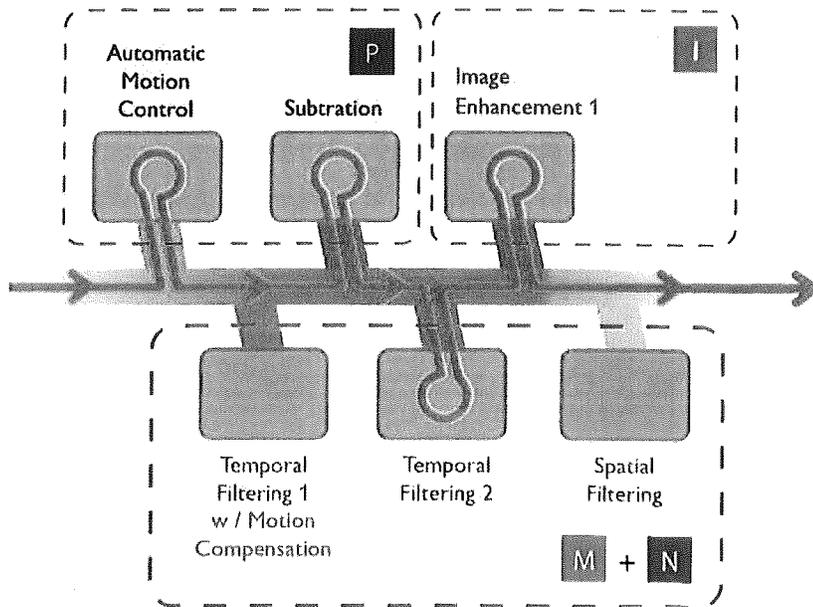
Figure 12: Illustration of the flexible digital imaging pipeline. In this imaginary example, the image goes through the subsequent processing steps of AMC, subtraction, temporal filtering and image enhancement. The letters P, M, N and I refer to the modules mentioned in Figure 4.
