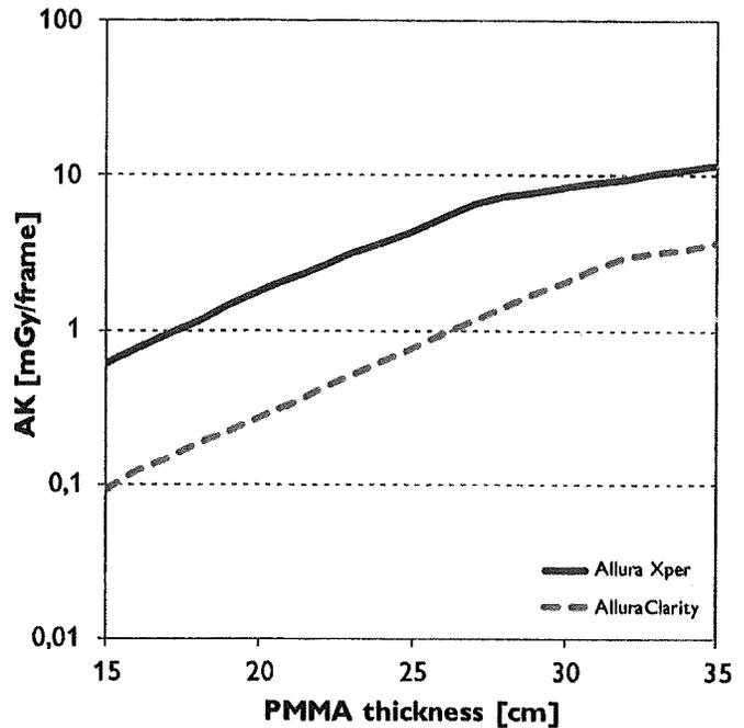
Figure 20: Neuro DSA Cerebral 2 fps patient dose comparison measured with an SID of 1 m for the largest detector format, measuring point is the PERP. Measurements have been performed on two separate FD20 systems (AlluraClarity and Allura Xper). Typical equivalent water thicknesses for interventional neuroradiology are around 23.7 cm with a standard deviation of 1.9 cm.
