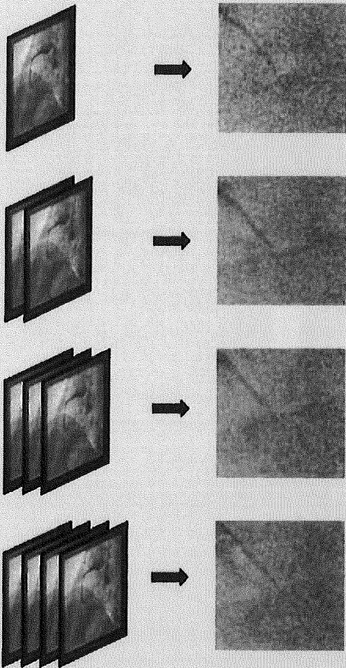
Figure 7 Example of temporal noise reduction. The noise is filtered by averaging over several frames. The signal is aligned (motion compensation) and then averaged. From top to bottom, the effect on the noise of using more images is shown.
