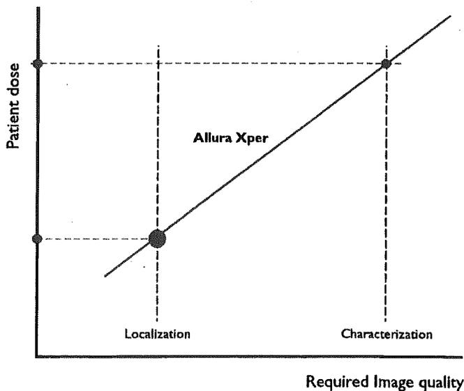
Figure 2: Graph of the relationship between IQ and patient X-ray dose for the Allura Xper. The positions for localization and characterization were chosen arbitrarily, and will be different for each application. Patient thickness and projections will also affect the graph.
